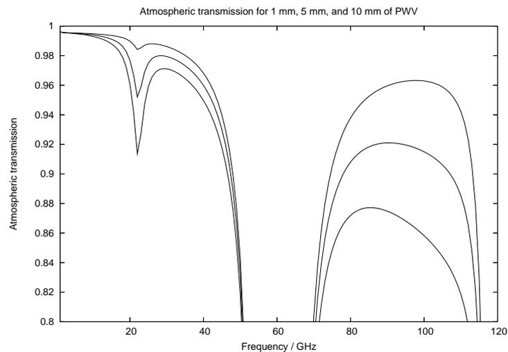
**Figure 3:** Atmospheric transparencies between 1 GHz and 120 GHz for values of precipitable water vapour (PWV) of 1 mm, 5 mm, and 10 mm. The higher the PWV, the lower the transparency.
