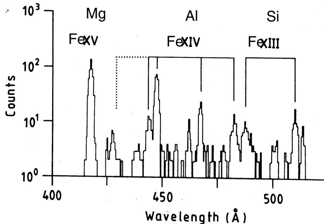
**Figure 1.** Delayed beam-foil spectrum of Fe. The intercombination lines in Fe xv, Fe xiv and Fe xiii are indicated. A dotted line marks the calculated location of the weak  $^2P_{1/2}-^4P_{3/2}$  transition in Fe xiv.
