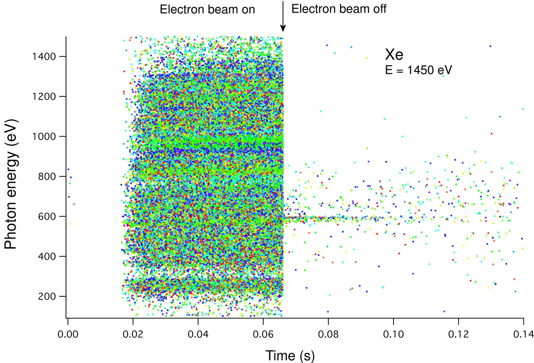
XRS microcalorimeter data recorded at the LLNL EBIT with a 140 ms trap cycle.
