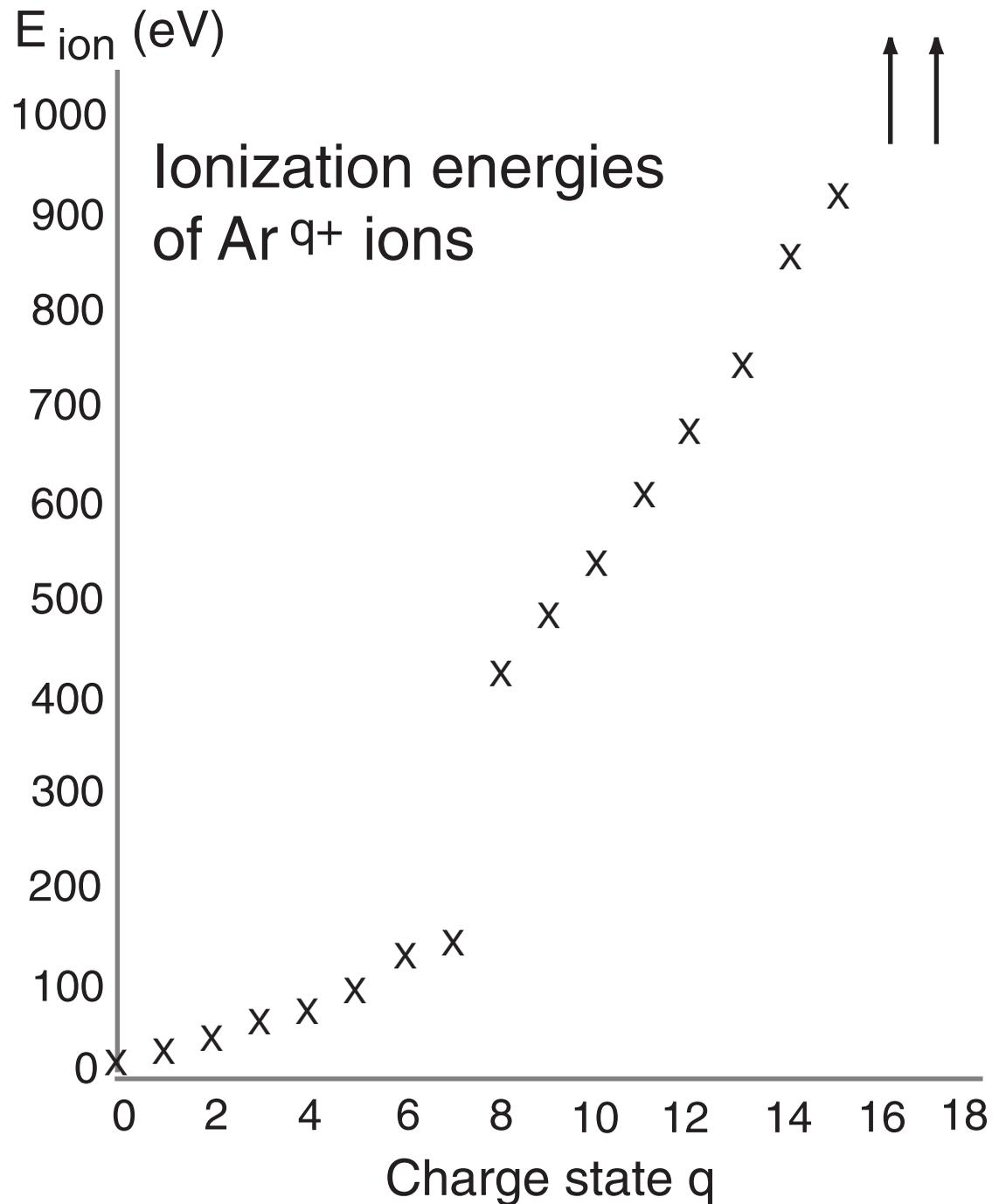
It is easy to reach any charge state of ions in an electron beam ion trap, by adjusting the electron beam energy.
